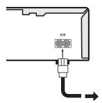
1 Use the supplied power cable to connect this recorder to a power outlet.
